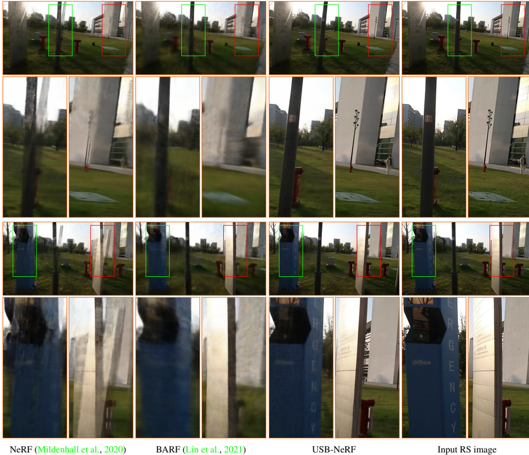
Figure 10: Qualitative comparisons on real-world datasets captured by a Canon camera. The camera exhibits forward and backward motion, which challenges both NeRF and BARF to recover the true underlying 3D scene representation. Our method recovers the correct global shutter images. Note the camera is not parallel to the ground during capture.
