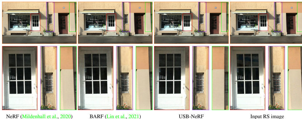
Figure 11: Qualitative comparisons on real-world datasets captured by GoPro HERO6. The images are captured on a moving tram in constant direction. It demonstrates that even both NeRF and BARF can render clear images, the recovered scene is distorted. Our method can correctly un-distort it.
